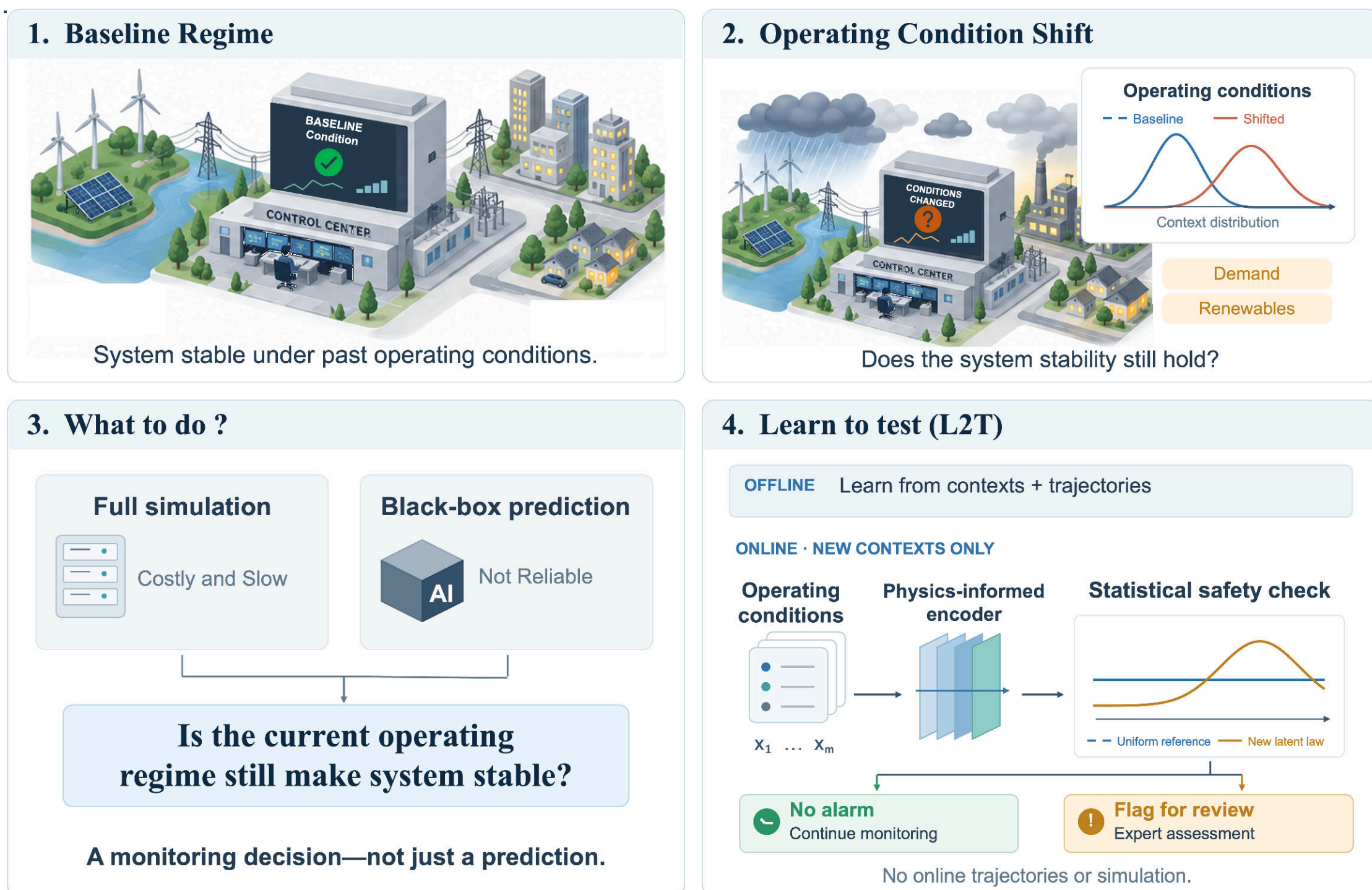
Figure 1. Simulation is too slow and a black-box predictor unreliable off-distribution, so L2T turns the question into a statistical check on new contexts alone — focusing expert attention where the assessment needs review .
